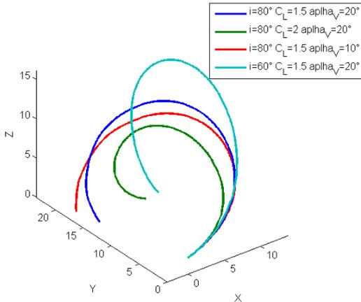
Figure 9: Boomerang trajectories for different initial parameters
