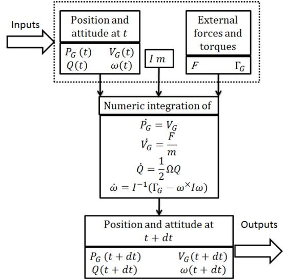
Figure 8: Numerical integration inputs and outputs
