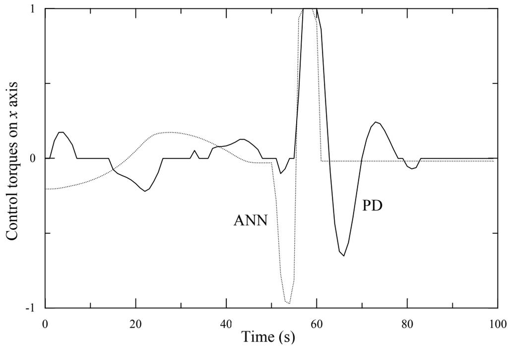
Fig. 4 – Control torque of the ANN and PD controllers, in the  $x$  axis.
