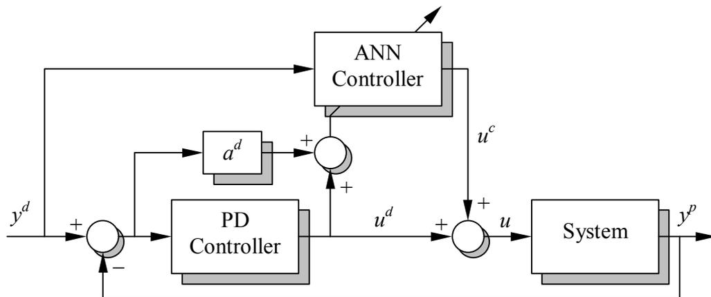
Fig. 2 – Feedback error learning control with acceleration threshold.
