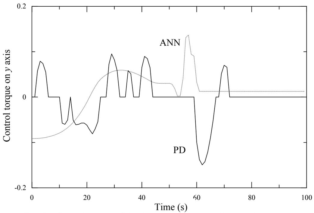
Fig. 5 – Control torque of the ANN and PD controllers, in the  $y$  axis.
