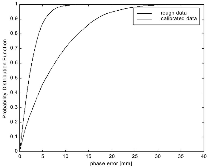
**Fig. 7 – Probability Distribution Function of Error at Single Difference Before and After Calibration**
