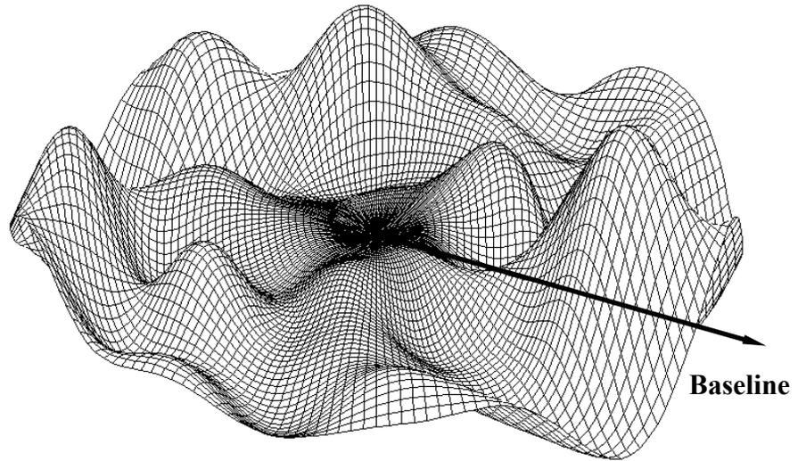
**Figure 4 Multi-path Error Modeled by Spherical Harmonic Series Based on Empirical Data**
