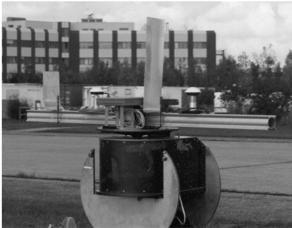
**Figure 2 GPS Ground Experiment with Multi-path Plates**
